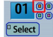
To assign a channel to be part of a fixture group, press one of the buttons in the upper right corner of the channel. There are four independent fixture groups indicated by the button color.
