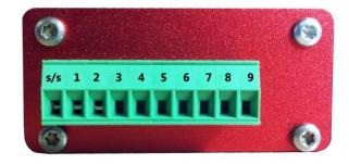
Trigger inputs wired for "Sinking" or "NPN" configuration. Sink/Source (s/s) terminal wired to 9 to 24vdc. Switch provides ground signal when closed.
